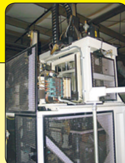
Automated Stator Wave Winder
