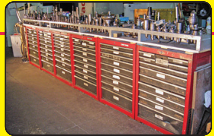
Partial View, Tooling Cabinets and 40 Taper CNC Holders
