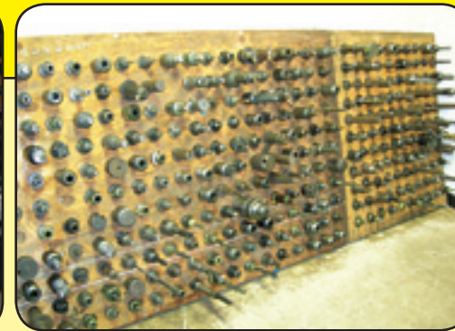
Partial View, 40 and 50 Taper Devlieg Holders (1,000+ Available)
